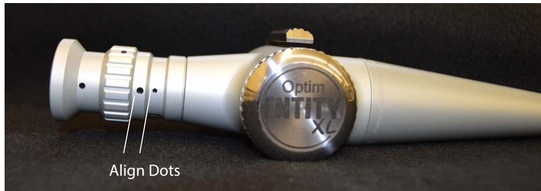
Figure 6. Alignment of Black Focus Ring Marks
