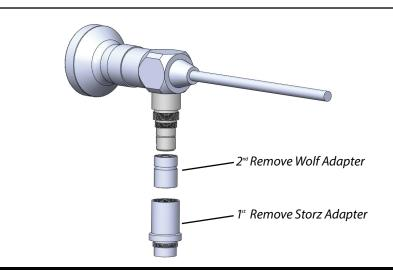
Rigid Endoscope with provided adapters attached
