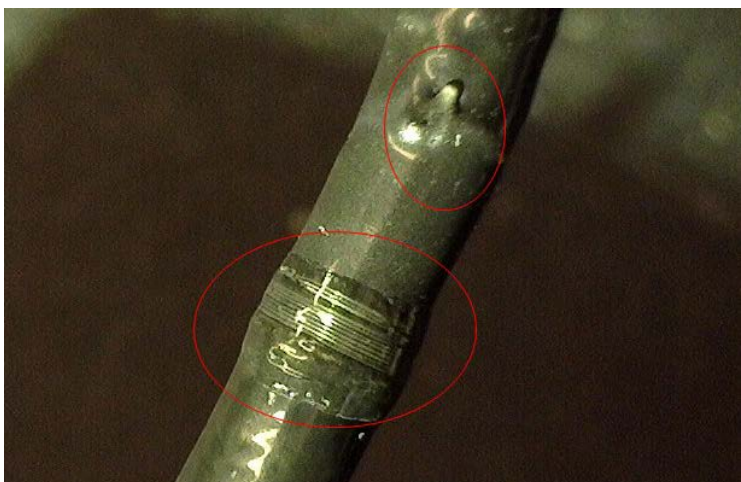
Improper material used, causing holes and tears
