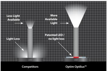
Optim's unique LED light source to fiber light guide coupling technology, Optilux™, in the FreedomView® Videoscope brings unmatched illumination to the end of the scope, where it counts.
